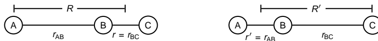
Figure 1: The ABC collinear system in the reactant (left) and product (right) arrangement. Reactant ( R , r ) and product ( R' , r' ) Jacobi coordinates are shown together with the process BL coordinates r_{AB} and r_{BC} .
